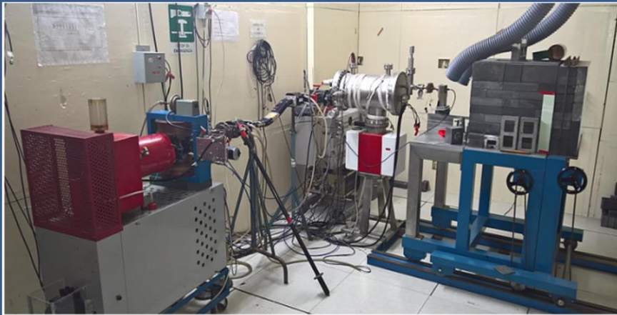
REX: Removable Electron to X-ray source (Max energy: 5 MeV)
