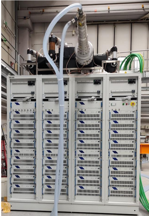
The INFN solid state ampli prototype (200kW, 175 MHz , 62% power efficiency)
