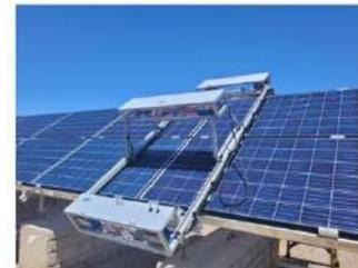
Fig 5. Image of the first prototype of the PV Array Inspection Robot placed on a PV array.
